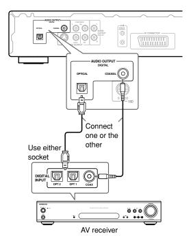
For an optical connection, use an optical cable (not supplied) to connect the "OPTICAL DIGITAL AUDIO OUTPUT" jack to an optical input on your AV receiver.
